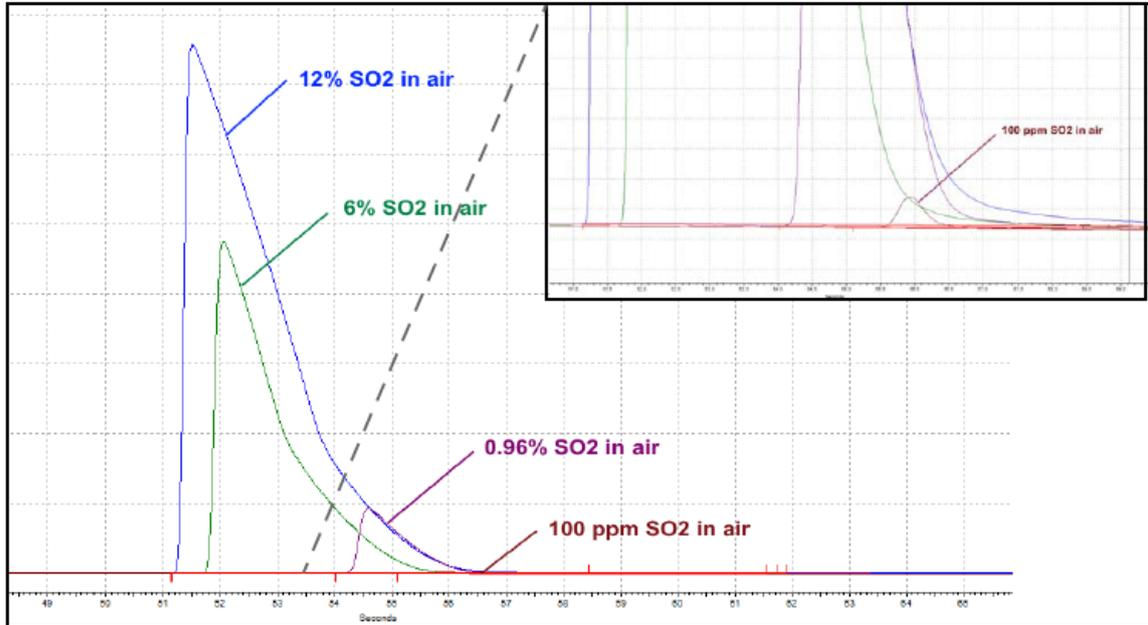
Figure 3 Calibration curve for SO<sub>2</sub>
