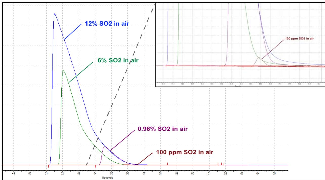
Figure 3 Calibration curve for SO<sub>2</sub>
