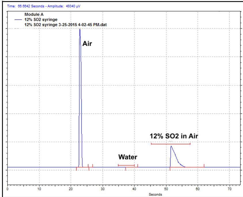
Module: 12 m Rt-Q-Bond column, Variable Volume Injector, TCD
