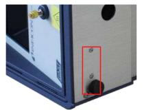
*6* Mount the gas-liquid separator for the 2-module chassis as shown. Hold the gasliquid separator so that the slots on the gas-liquid separator align with the holes on Micro GC Fusion.
