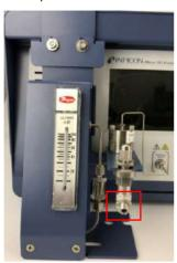
*21* Install a user-provided 1/8 in. sample line with the female Swagelok fittings preinstalled.
