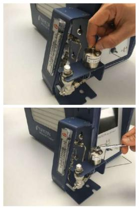
**12** Put the 5/16 in. Swagelok nut (PN 059-0696) and the 1/16 in. ferrule set (PN 059-0697) on the other end of the sample tube.
