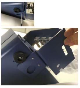
8 Loosen the top two nuts on the mounting bracket.
