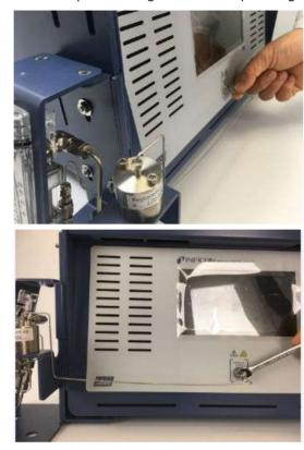
**12** Insert the 1/16 in. sample tubing with the Swagelok fittings onto the instrument sample inlet. Tighten 1/2 turn past finger-tight using the 5/16 in. wrench.
