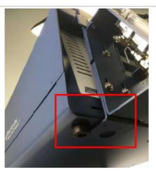
7 Put the two M3 screws (PN B3079191X) through the two small holes in the mounting bracket bottom and into the instrument chassis bottom with a 2.0 hex driver.
