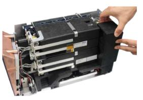
*11* Replace the side foam. Ensure the dovetail joint is oriented as shown.
