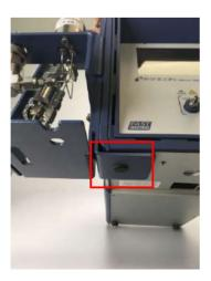
*8* Adjust the nut position to remove the gap between the mounting bracket and the chassis top.
