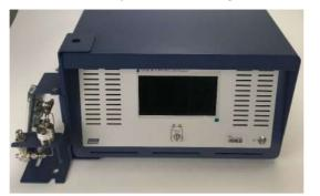
*8* Adjust and tighten all the nuts using a 3/8 in. wrench to fix the mounting bracket on the instrument chassis.
