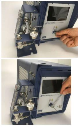
14 The pressure reducer and gas-liquid separator installation is complete. Reconnect the power cable, the Ethernet cable and the carrier gas lines.
