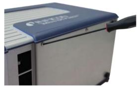
*6* Turn Micro GC Fusion back to its upright position. With finger tips, grasp the bottom lips of the housing on both sides, carefully pull them apart and lift the housing off Micro GC Fusion.
