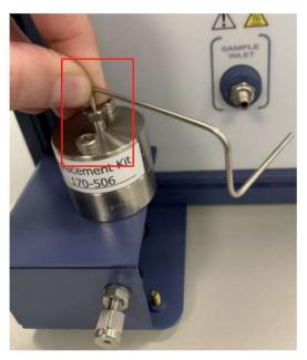
11 Place the 1/16 in. nut (059-0696) and the ferrule set (059-0697) onto the end of the sample output tubing going to Micro GC Fusion.
