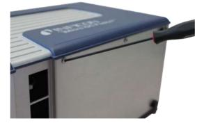
*6* Turn Micro GC Fusion back to its upright position. With finger tips, grasp the bottom lips of the housing on both sides, carefully pull them apart and lift the housing off Micro GC Fusion.
