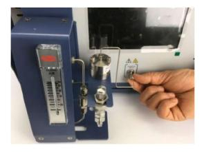
18 Tighten 1/2 turn past finger-tight using the 5/16 in. wrench.
