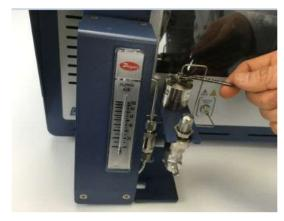
16 Put the 5/16 in. Swagelok nut (PN 059-0696) and the 1/16 in. ferrule set (PN 059-0697) on the other end of the sample tube.
