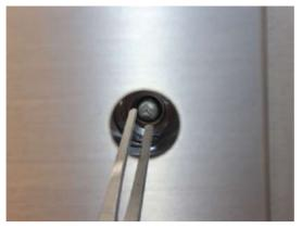
**7** Use forceps to place a new filter into the unit. Ensure the flat side of the filter faces the forceps.
