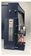
**17** Connect a vent line to the vent fittings using 1/8 in. Swagelok fittings. Run the exhaust to a fume hood or other designated area for hazardous waste disposal.
