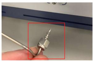
11 Connect the sample output tubing from the gas-liquid separator to the Micro GCFusion sample inlet and tighten using a 5/16 in. wrench.
