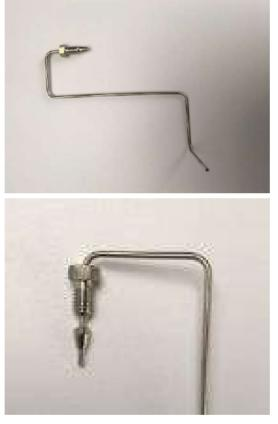
**14** Insert the sample tubing with the Valco fittings into the fitting detail on the Genie filter. Push the tubing all the way into the detail, so that it seats firmly. Manually turn the nut into the detail until it is finger tight.
