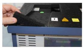
14 With finger tips, grasp the bottom of the housing cover and gently pull apart.Position the cover over Micro GC Fusion and lower to replace the housing cover back on Micro GC Fusion.
