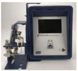
*10* Put the Valco ferrule (PN 059-0335) and the nut (PN 059-0336) on the inlet tube.
