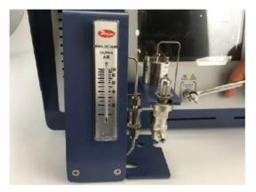
19 The pressure reducer and gas-liquid separator installation is complete.Reconnect the power cable, the Ethernet cable and the carrier gas lines.
