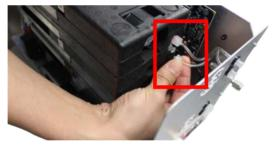
14 Remove the GC module by lifting it and pulling it sideways out of the chassis.
