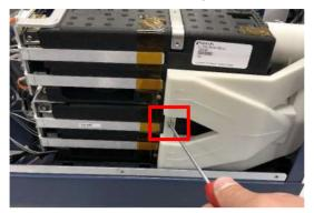
⇒ For modules A/B, remove the retaining screw holding the JP-100 in place with the 2.5 mm ball point hex wrench.
