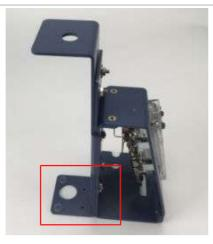
**5** Set the five nuts on the mounting bracket to the positions shown. If the nut positions need adjustment, relax the nuts, adjusting the mounting bracket and retighten the nuts using a 3/8 in. wrench.
