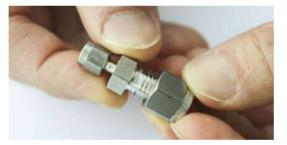
5 Insert the 1/4 in. tube fitting on the 3 L sample bag into the 3/16 in. end of the SSAdapter for the Sample Bag and screw clockwise until finger tight.
