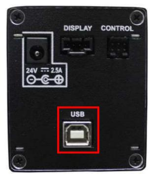
*18* Connect the Manual Controller to the back of the Valco stream selector to manually control the internal actuator.
