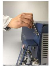
*9* Put the Valco ferrule (PN 059-0335) and the nut (PN 059-0336) on the inlet tube.
