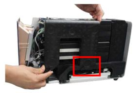
12 With finger tips, grasp the bottom of the housing cover and gently pull it apart.Position the cover over Micro GC Fusion and lower it down over the housing to replace the housing cover back on Micro GC Fusion.
