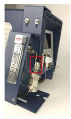
*16* Install a user-provided 1/8 in. sample line with the female Swagelok fittings preinstalled.
