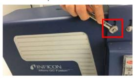
*9* Tighten all nuts with a 3/8 in. wrench to fix the bracket on the instrument chassis.
