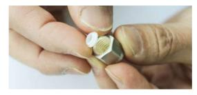
⇒ Place the Teflon front ferrule into the nut with the narrow end facing outwards.
