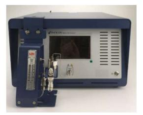
**20** Before connecting the pressurized sample to the device, close the metering valve by turning the dial fully clockwise to ensure no sample flow through the device when the pressurized sample is connected.
