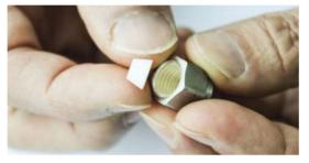
*4* Screw the 3/16 in. stainless steel nut with the Teflon ferrules back into the reducing union (PN 059-0298).
