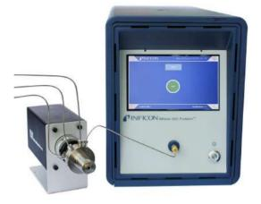
A Valco stream selector is connected to and controlled by Micro GC Fusion via a USB connection on the back of the instrument. The proper USB cable is provided with the Valco stream selector.
