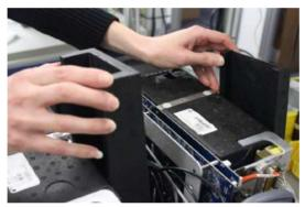
**12** Replace the top foam by grasping one front corner and the opposite back corner, and pressing straight down.
