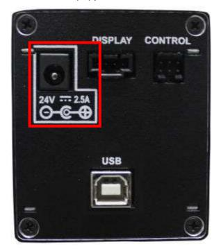
**17** Connect the USB Type B connector of the USB cable to the back of the Valco stream selector. Connect the USB Type A connector of the USB slot in the back of Micro GC Fusion.
