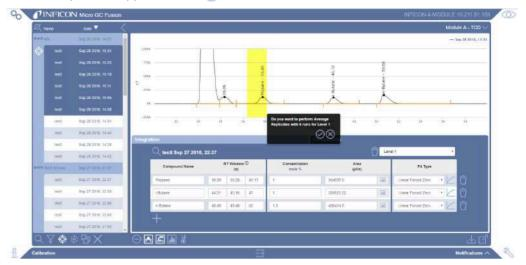
4 The Area (μV) column will automatically populate with the new area counts for all compounds in the run. The name of the calibration will be replaced with the currently selected run. When using average replicates, one of the data files used in the calculation will be used as the reference chromatogram for the calibration.
