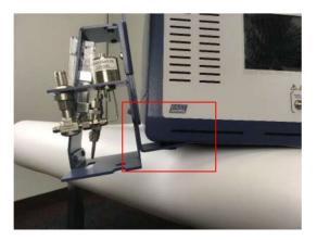
7 Push the top of the mounting bracket towards the instrument until it fits tightly.
