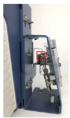
*18* Slowly open the dial to allow the sample to flow through the device. Check the flow indicated on the flow gauge and ensure it is less than 100 mL/min.
