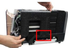
8 Remove the rear foam by pulling it sideways out of the instrument back.
