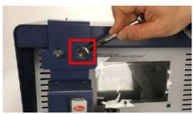
**12** Adjust and tighten all the nuts using a 3/8 in. wrench to fix the mounting bracket on the instrument chassis.
