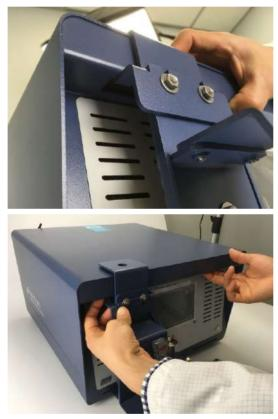
**11** Tighten the two nuts using a 3/8 in. wrench to ensure that bracket E does not fall off.
