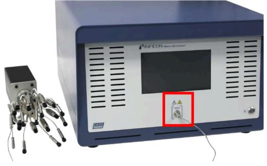
16 Plug the DC power connector on the power supply into the back of the Valco stream selector. Connect the AC power connector on the power supply into a 100-240V (ac) power source.
