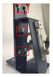
*6* Clamp the mounting bracket onto the left side of the instrument, with the large hole on the bottom of the mounting bracket fitting into the left front foot of the instrument.
