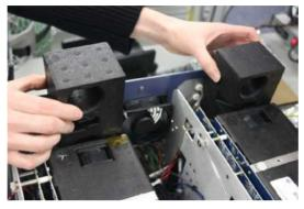
*11* Replace the side foam. Ensure the dovetail joint is oriented as shown.
