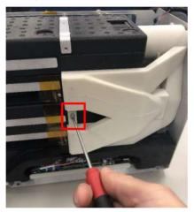
9 Slide the JP-100 up and out of the instrument.
