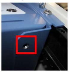
*6* Secure the instrument on the brackets with the provided flat Phillips head screw (PN 090-062).
