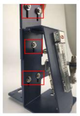
*6* Clamp the mounting bracket on the instrument front, with the mounting bracket bottom to the right side of the instrument left front foot.
