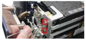
*13* Loosen and remove the venting connectors at the rear of the GC module by turning counterclockwise.
