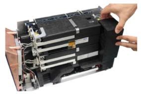
9 From the left side of the Micro GC Fusion chassis frame, use a Phillips head screwdriver to loosen the two captive screws that hold the GC module. To remove the lower GC module, loosen the two captive screws.
