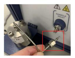
**12** Connect the sample output tubing from the gas-liquid separator to the Micro GC Fusion sample inlet and tighten using a 5/16 in. wrench.
