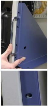
⇒ Thread the oval head screw (PN 090-077) through the washer (PN 070-2028) as shown, then screw the bracket into the retainer nut.
