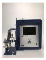
7 Ensure the bottom mounting bracket hole is fitted into the lower left chassis foot.
