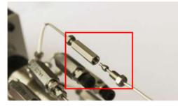
8 Connect the 1/16 in. OD stainless steel tubing to the OUT TO GC union.
