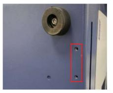
**5** Mount the gas-liquid separator for the 4-module chassis as shown. Hold the gasliquid separator so that the slots on the gas-liquid separator align with the holes on Micro GC Fusion.
