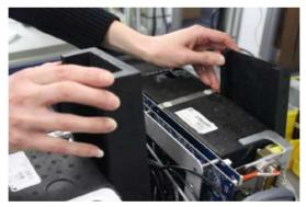
10 From the left side of the Micro GC Fusion chassis frame, use a Phillips head screwdriver to loosen the two captive screws that hold the GC module. To remove the lower GC module, loosen the two captive screws.
