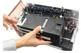
**15** Repeat the same procedure (steps 9-14) to remove the lower module, if necessary.
