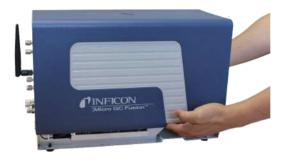
7 Remove the side foam by pulling it sideways to free it from the dovetail joint at the bottom.
