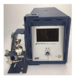
**15** Before connecting a pressurized sample to the device, close the metering valve by turning the dial fully clockwise to ensure no sample flow through the device when the pressurized sample is connected.
