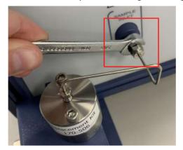
13 Tighten the Valco fitting on the gas-liquid separator using a 1/4 in. wrench.
