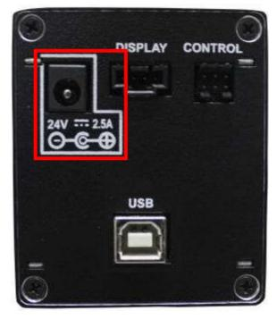
13 Connect the USB Type B connector of the USB cable to the back of the Valco stream selector. Connect the USB Type A connector of the USB slot in the back of Micro GC Fusion.
