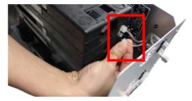
**4** Use a 2.5 mm ball point hex driver to replace the two carrier gas manifold screws onto the GC module. Tighten them until they are snug.
