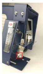
**17** Connect a vent line to the vent fitting using 1/8 in. Swagelok fittings. Run the exhaust to a fume hood or other designated area for hazardous waste disposal.
